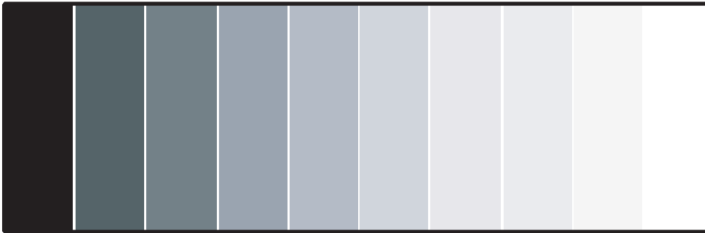
Figure 4-4. Typical Gray Bar Pattern for Adjusting Contrast
